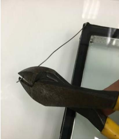
Figure 1: Cutting Tube ½" From End
