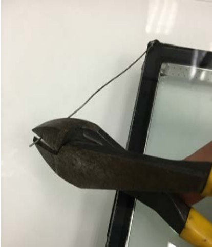
Figure 1: Cutting Tube 1/2" From End
